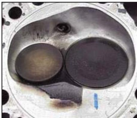
terns in or around the valve pocket...especially at high valve lifts. Dye sprayed briefly into ports during air bench analysis can reveal areas of fuel collection (separation) and distribution; patterns frequently similar to those seen after combustion patterns are established by running the engine.
