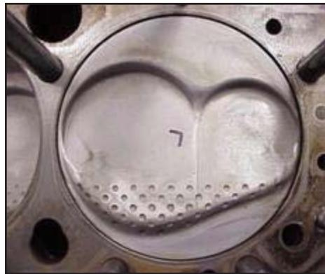
To aid mixture quality {reduce air/fuel separation} just past piston dome edges, dimples can be placed to assist mixtures in turning over the pad and around toward the exhaust valve (counterclockwise mixture motion direction shown).
