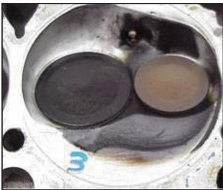
In this clockwise motion pattern, note the "clean" area on the chamber's back wall, indicating air/fuel impingement and subsequent separated fuel from the air. The low-pressure area just past the spark plug encourages fuel to collect, leading to a fuel rich condition, as evidenced by the dark area. Separated fuel further "washes" past the exhaust valve, burning to a rich condition past this valve and toward the intake valve.
