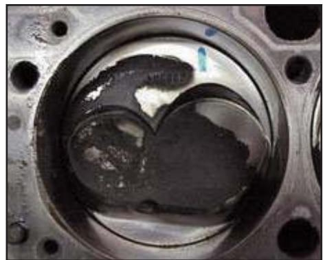
Here's clockwise pattern clearly revealing mechanical air/fuel separation across the intake valve pocket, behind the compression dome and over the quench area (deck). Wide ranges of air/fuel ratios were present, including very wide areas across the dome's crown and especially inside the exhaust valve notch. From this photo alone, it should be evident how "ranges" of air/fuel mixture can exist in a given combustion space undesirably so, too.
