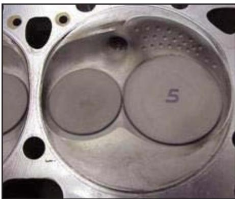
This is an alcohol-fuel small-block Chevrolet V8 combustion chamber showing uniform combustion flame patterns, aided by the dimpled places on the back wall in an area typically "washed" with fuel.
