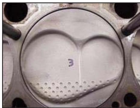
Look closely at this image and you'll note the slightly darker area from about 3:00 o'clock to 6:00 o'clock (counterclockwise mixture motion direction). This suggests additional dimples should be placed in the area of the intake valve's relief, aiding mixture quality of air and fuel passing over the crown and passing the piston's deck surface below (as seen in this view) the exhaust valve relief.
