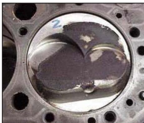
This piston is in trouble. Note mechanical separation of air and fuel across intake valve relief and on backside of piston crown from one side to the other. Heavy buildup of carbon on top of piston crown indicates excessively rich mixture burn in this area. Mixture motion is counter-clockwise.
