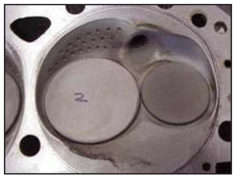
This image indicates close piston-tohead proximity in the quench area (lower left-hand portion of the photo) and a slightly richer condition (compared to the remainder of the chamber's color) along the edges of this quench condition – not uncommon nor necessarily undesirable when running very tight deck clearances.
