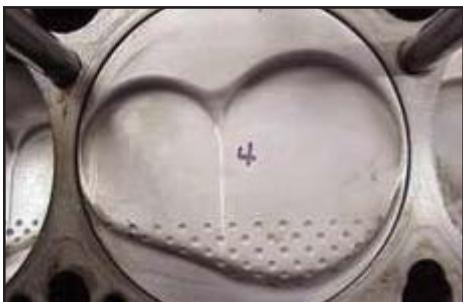
In this clockwise motion pattern, note the absence of a "clean" area in the intake valve relief. Radiusing this edge helps reduce the "edge" effect and cause of separated air and fuel in this area.
