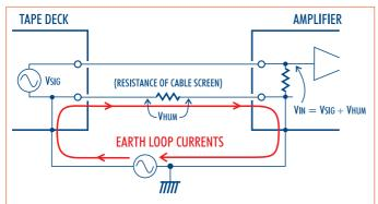
Fig.2: When there is an earth loop, AC currents induced in it can inject hum into the signal circuits via the screening braids of the interconnecting cables.
