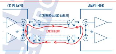
Fig.3: Even a pair of stereo interconnecting cables can create an earth loop...
