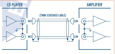
Fig.4: One solution is to use 'twin screened' leads with a single earth connection.
