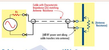
Fig.3: A transmitter or other source of RF feeding power to an antenna, via a coaxial cable or other transmission line. Here's where impedance matching IS important...
