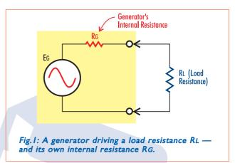
impedance. And the idea of matching the load and generator resistance became one of matching the source and load impedance — *impedance matching*.
