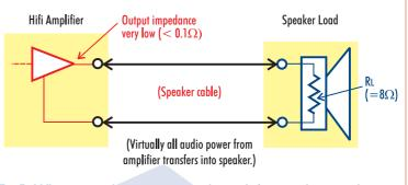
Fig.5: When a speaker is connected to a hifi amp, the impedances are NOT matched.
