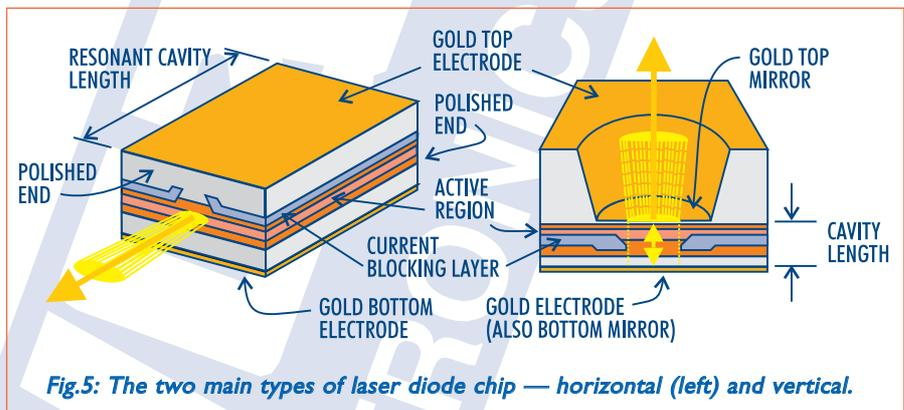
**Fig.5: The two main types of laser diode chip — horizontal (left) and vertical.**
