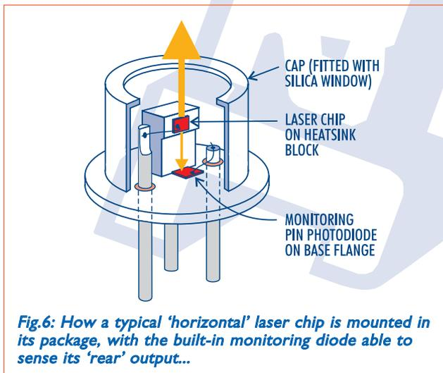
**Fig.6: How a typical 'horizontal' laser chip is mounted in its package, with the built-in monitoring diode able to sense its 'rear' output...**
