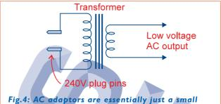
stepdown transformer in an 'enlarged plug' case.
