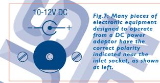
With DC power adaptors which use the interchangeable plug system, the plugs are usually capable of being connected to the adaptor cable either way around. This makes it very easy to set the plug for the correct polarity. However if you use an adaptor which only comes with a single fixed plug, and its polarity turns out to be wrong for your equipment (Murphy's Law strikes again!), you'll probably have to cut the plug off the cable and fit another plug with the correct polarity.
