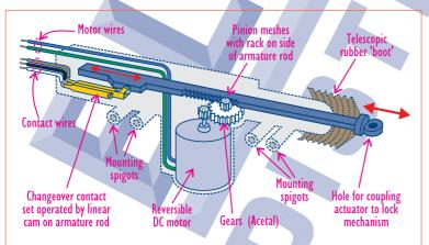
Fig. 1: What's inside a master actuator. A slave actuator is virtually identical except that it lacks the set of contacts used to monitor the position of the armature rod.
