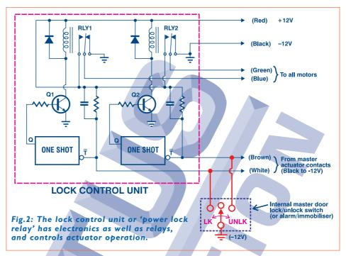
Even better, brief short connections of either oneshot trigger input to -12V can also operate all of the actuator motors, and this is how a 'master door control' switch inside the car works. It's also how a burglar alarm or immobiliser can control the door locking system, simply by using relay contacts to connect either one-shot input to -12V briefly.
