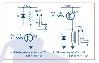
If our relay has a coil resistance of say  $180\Omega,$  so that it draws say 67mA at 12V, we'd need to reduce R1 to say  $8.2k\Omega,$  to increase the base current to about 1.4mA. Conversely if the relay coil is  $360\Omega$  and draws only 33mA, we could increase R1 to  $15k\Omega,$  giving about 0.76mA of base current. Each time we go for about twice the relay coil current divided by Q1's hFE — get the idea?
