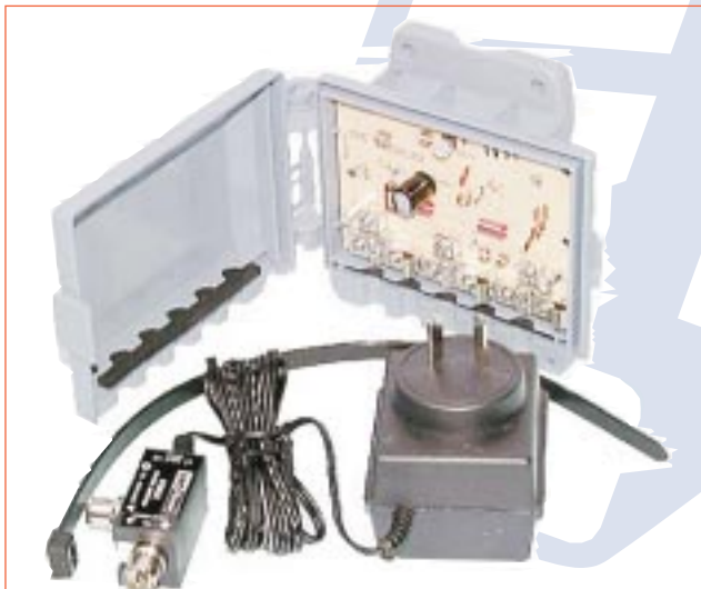
Masthead amps have quite specific uses, as we explain in the text. This one is the GME Kingray MHW34GP (Jaycar LT-3290).
