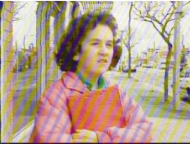
Fig.8: The kind of effect you can get from EMI caused by a continuous radio signal, such as from a radio transmitter or diathermy. The coloured lines can be sloping either way, and at any angle.
