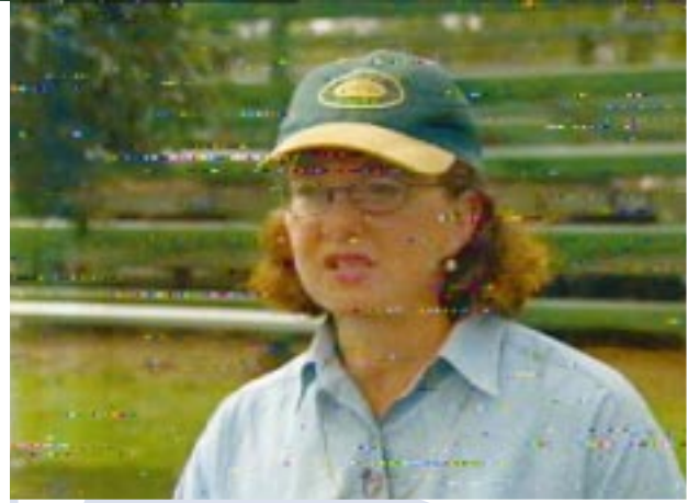
Fig.9: Another kind of EMI, caused by impulse noise from a power tool or food mixer. Corona discharge from high voltage power lines can look similar, but with the noise in horizontal 'bands'.
