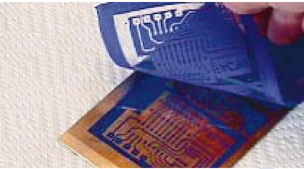
3. Place film emulsion down on blank board, then 'iron' to melt and transfer toner. Dunk in water...
